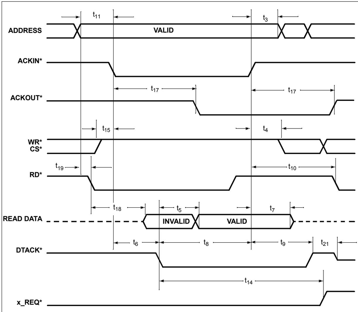
Figure 42. Unlocked Bus Interface Write Cycle, Intel®-Style Handshake
