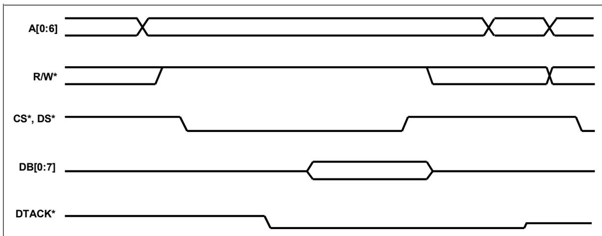
Figure 18. Typical Clocked Bus Interface
