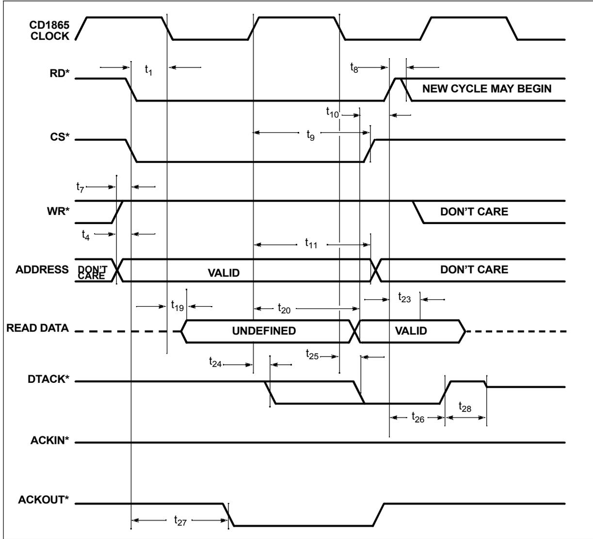
Figure 35. Clocked Bus Interface Service Acknowledgment Cycle, Intel®-Style Handshake
