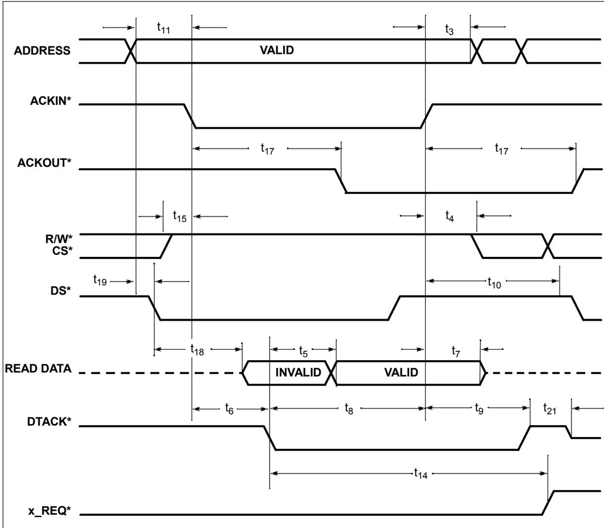
Figure 39. Unlocked Bus Interface Write Cycle, Motorola®-Style Handshake
