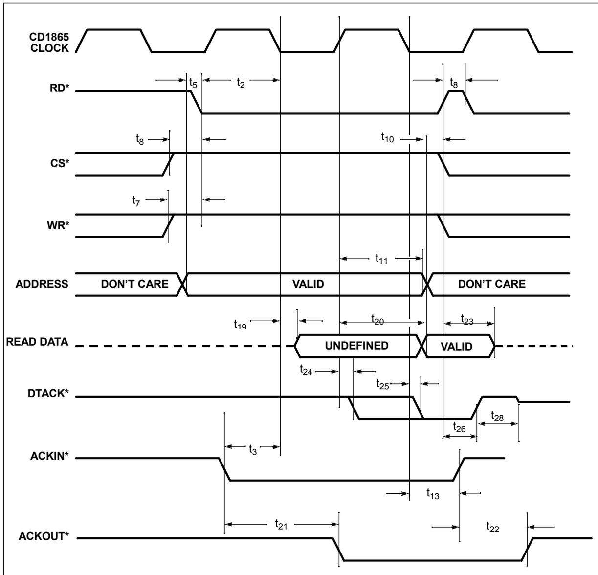
Figure 36. Clocked Bus Interface Write Cycle, Intel®-Style Handshake
