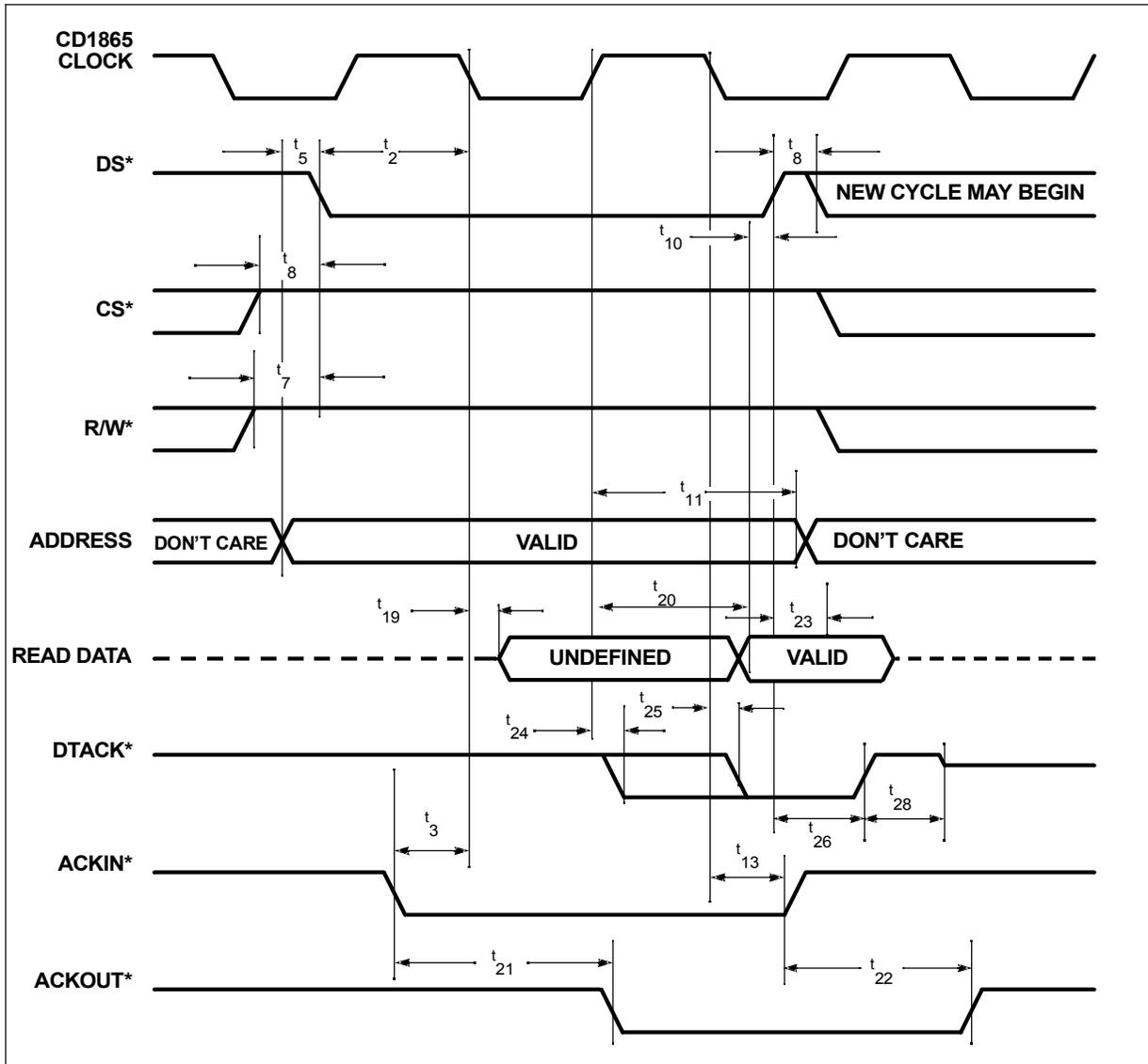
Figure 33. Clocked Bus Interface Write Cycle, Motorola®-Style Handshake
