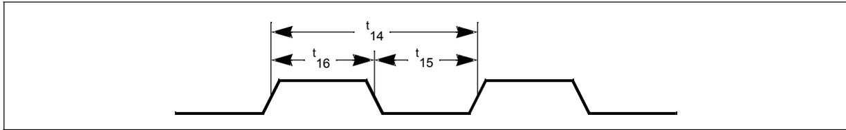
Figure 31. Clocked Bus Interface Read Cycle, Motorola®-Style Handshake
