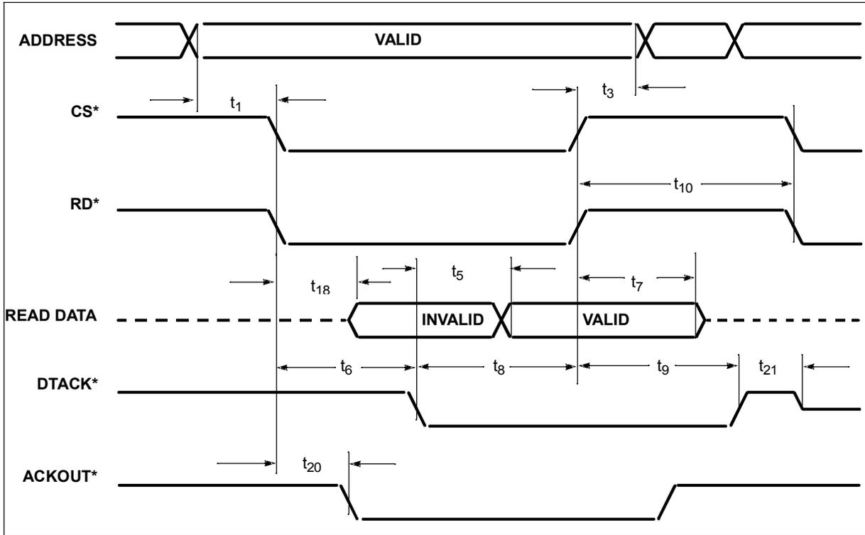
Figure 41. Unlocked Bus Interface Service Acknowledgment Cycle, Intel®-Style Handshake
