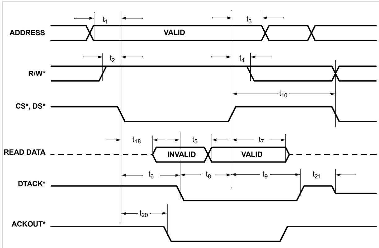
Figure 38. Unlocked Bus Interface Service Acknowledgment Cycle, Motorola®-Style Handshake
