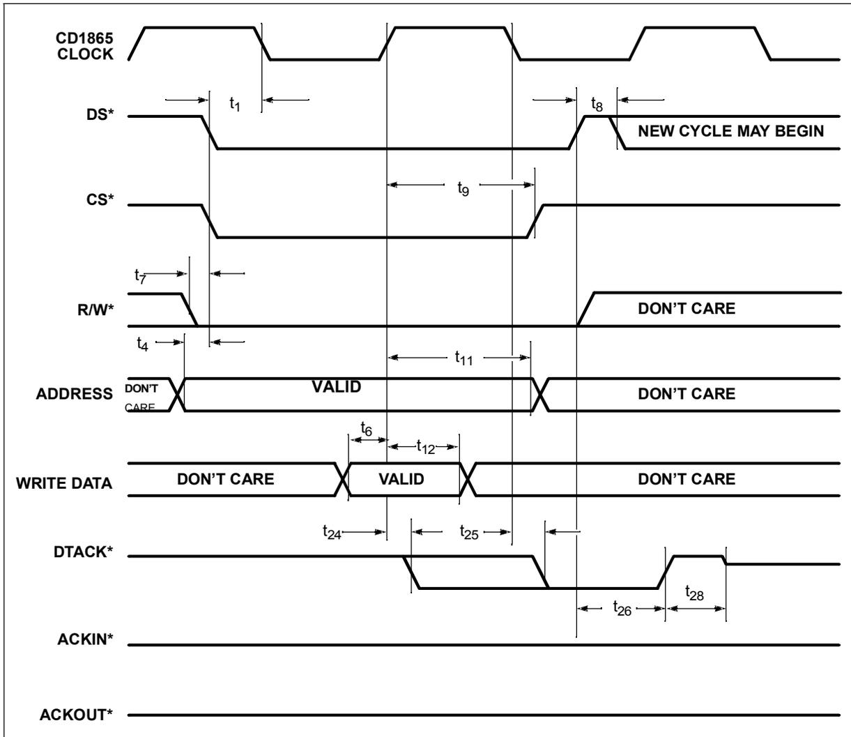
Figure 34. Clocked Bus Interface Read Cycle, Intel®-Style Handshake
