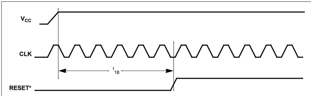
Figure 30. Clocked Bus Interface Clocks
